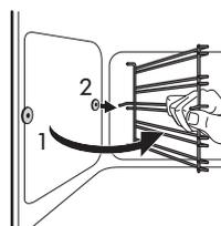
Pull the rear end of the shelf support away from the side wall and remove it.
