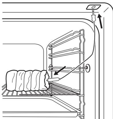
Make sure that the core temperature sensor stays in the meat and in the socket during the cooking.
