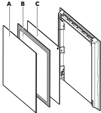
Make sure that you install the middle panel of glass in the seats correctly.
