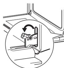
Lift and turn the levers on the two hinges.
