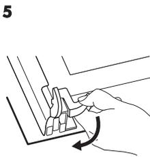
5 Release the locking system to remove the glass panels.
