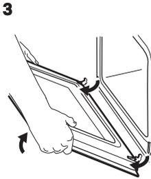
3 Close the oven door halfway to the first opening position. Then pull forward and remove the door from its seat.
