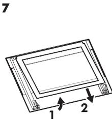
7 First lift carefully and then remove the glass panels one by one. Start from the top panel.
