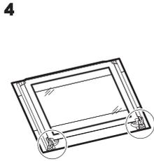
4 Put the door on a soft cloth on a stable surface.
