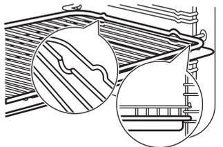
**i** Small indentation at the top increase safety. The indentations are also anti-tip devices. The high rim around the shelf prevents cookware from slipping.
