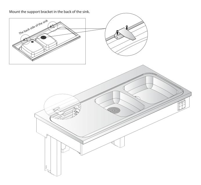
Fix the front edge of the sink at the left and right edges.
