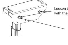
Loosen the locking screws (the inner, smaller screw) at all the motors. Adjust the inclination with the ex centre screw.
