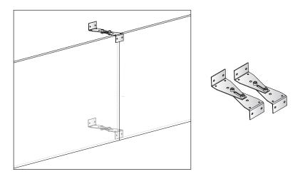
**4.14.4** Mounting of cover plates in corner, model 6201, 6202 and 6203.
